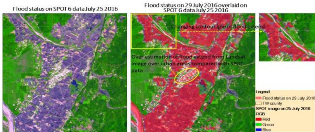
**Fig. 3** Flood status on SPOT 6 image and its comparison with flood status on Landsat data.
