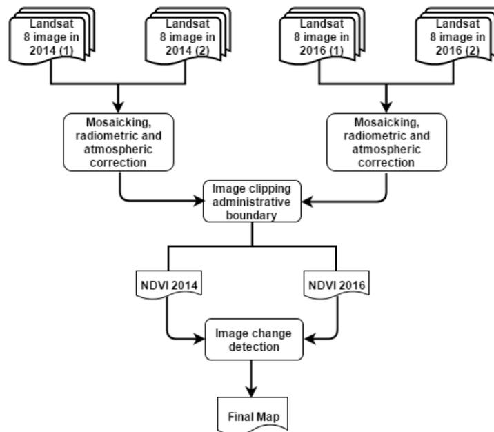
**Figure 5.** Data Processing Flow
